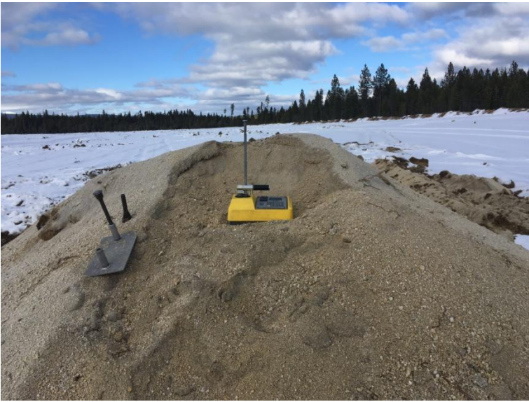
Figure 1: Exposed piles of homogeneous materials that required moisture testing. Upper imagine is a paleosol with high clay and organic contents. Lower imagine is pumice sands.
