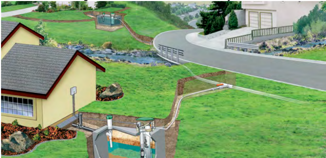
Figure 5.1 Effluent Sewer Collection System
