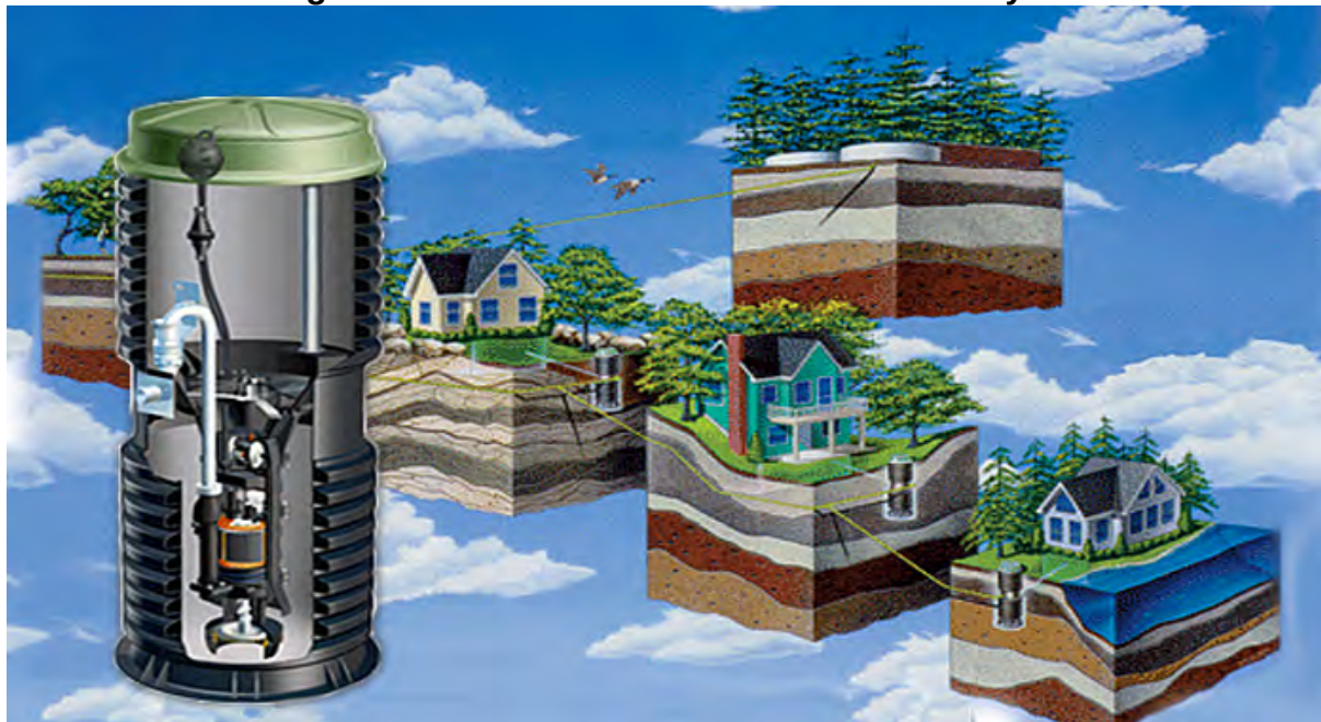
Figure 5.3 Low Pressure Sewer Collection System
