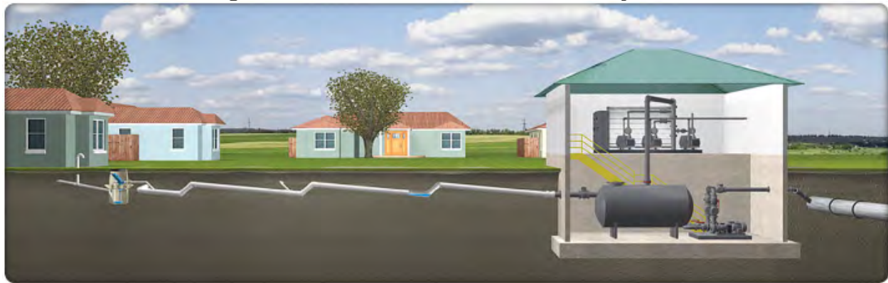
Figure 5.2 Vacuum Sewer Collection System
