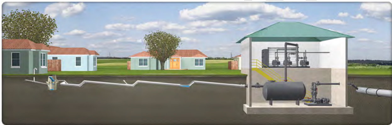
Figure 5.2 Vacuum Sewer Collection System
