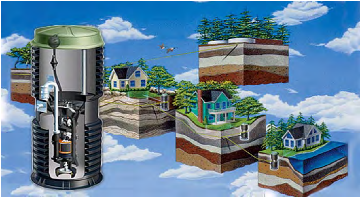
Figure 5.3 Low Pressure Sewer Collection System
