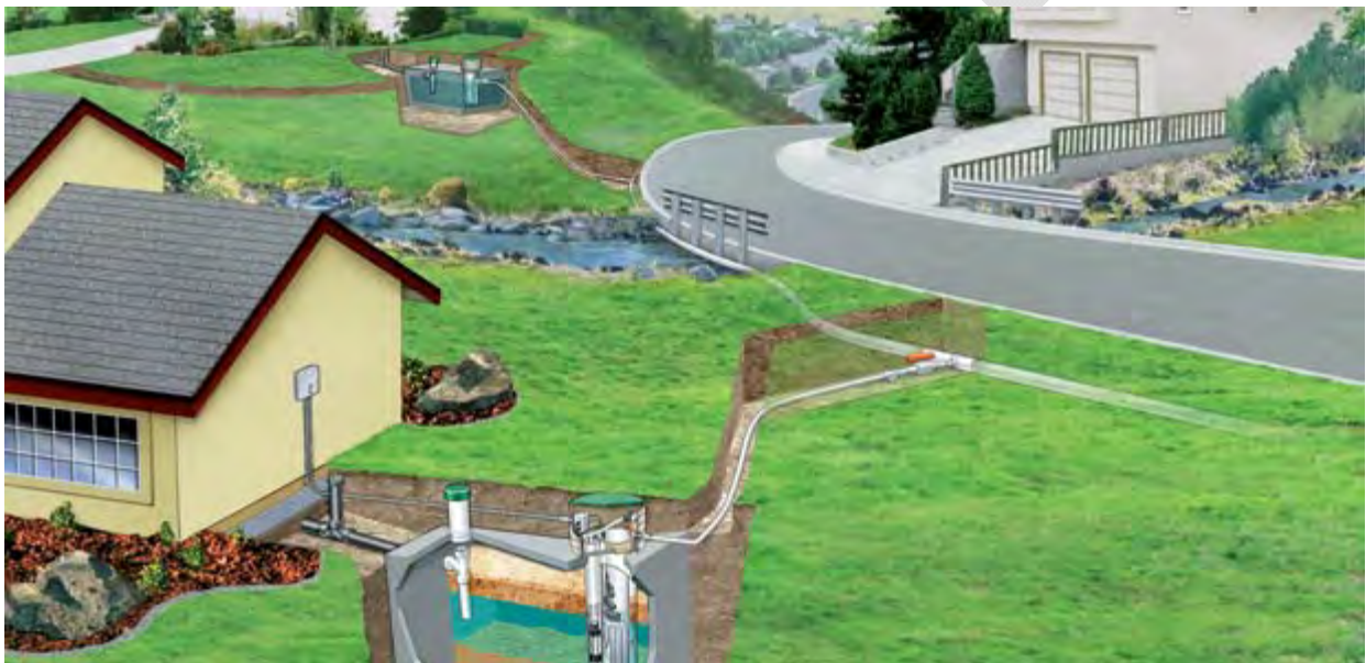
Figure 5.1 Effluent Sewer Collection System
